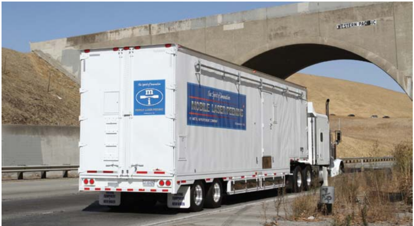
Figure 1. This MIC transportable laser system is en route to Palmdale, California for F-22 laser peening. MIC has a fleet of five mobile peening systems that can service marine, offshore oil and gas, petrochemical and aerospace repair and overhaul applications.
